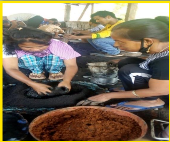
The powder mixed with tar and made into paste
