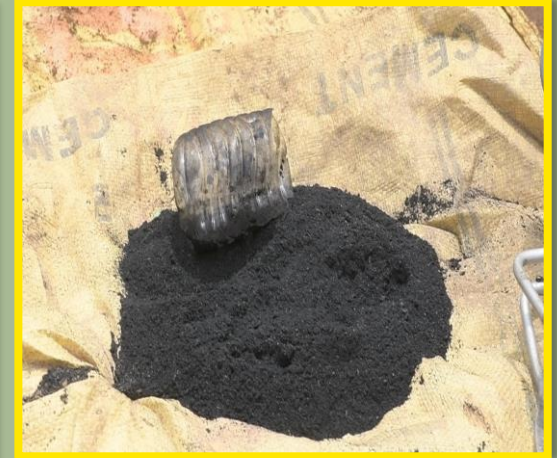
Carbonised is crushed into fine particles
